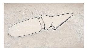
• Twist the other end of the coiled tubing (with the plastic quick disconnect) onto the plastic fitting in the silicone tip.
