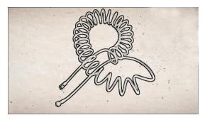
• Screw the metal fitting on the coiled tubing into the metal fitting on the main housing.
