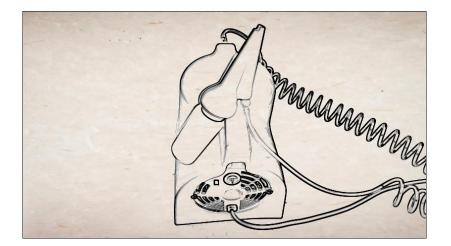
Rinsing the entire hand piece after each use will prevent clogging and insure top performance of the system. Picking away dried dental cleaner with a sharp tool will damage parts. Dried cleaner can be scrubbed away with water and a soft bristle brush. Routinely disinfect the tip with mild household cleaner or alcohol.
